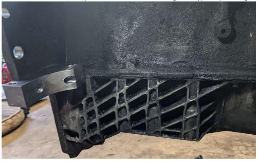
Locate the (2) M6 bolts and loosely mount the front starter brace to the engine block. Install your GM 6.2/6.5 starter as you would on a 6.2/6.5 diesel, using shims, if necessary. Attach the support bracket on the front and tighten the
