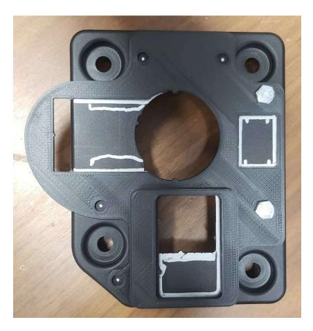
Use a Dremel or small rotary cutting tool to cut out the traced areas. Note that the bottom of the bezel doesn't need to be cut all the way thru. You only have to cut enough material to allow the 7/4-pin trailer plug receptacle to bottom out.
