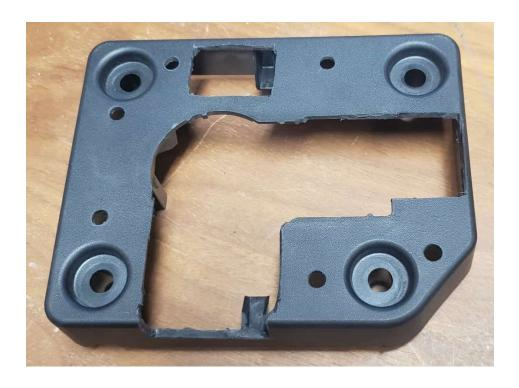
Take note of the 2 locating pins on the back side. You don't want to cut these off because they position the bezel on the bedside and help keep it from moving. You will have to clearance around them, but do not cut them clean off.
